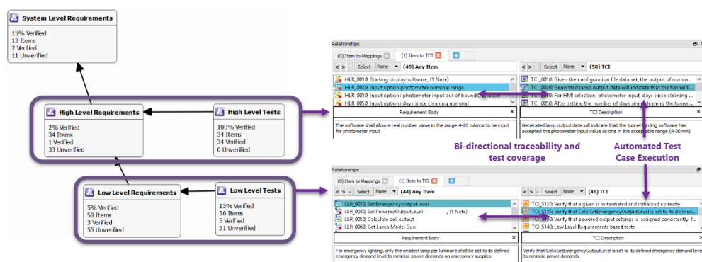
Figure 29: Performing requirement based testing. Test cases are linked to requirements and executed within the LDRA tool suite.
